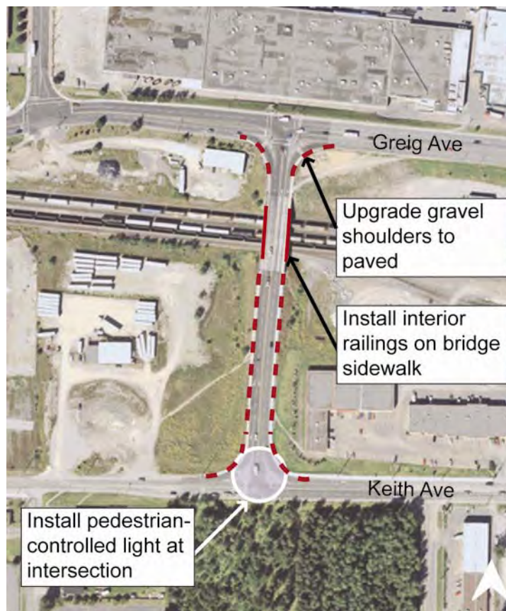
Figure 10. Recommended improvements to Sande overpass
