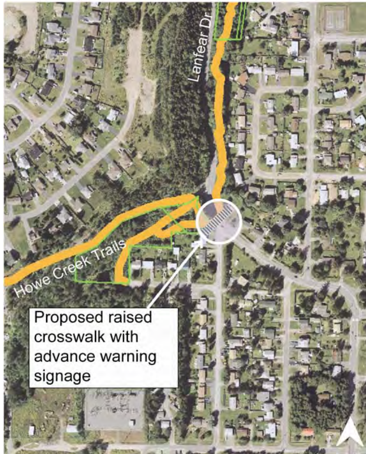
Figure 16. Recommendations for Lanfear Drive
