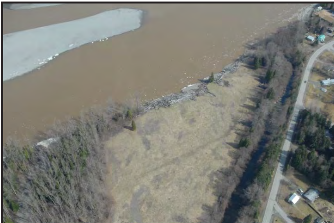
b) Looking upstream showing overbank debris deposited in the secondary channel which flows around the Regional District STP.
