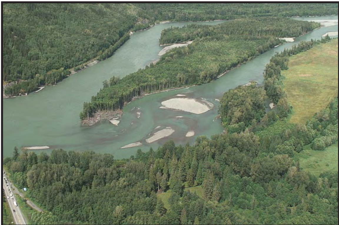
b) Looking upstream from the Highway 37 Bridge showing a locally eroding island, in-stream gravel storage and a cleared field with intermittent riparian vegetation.
