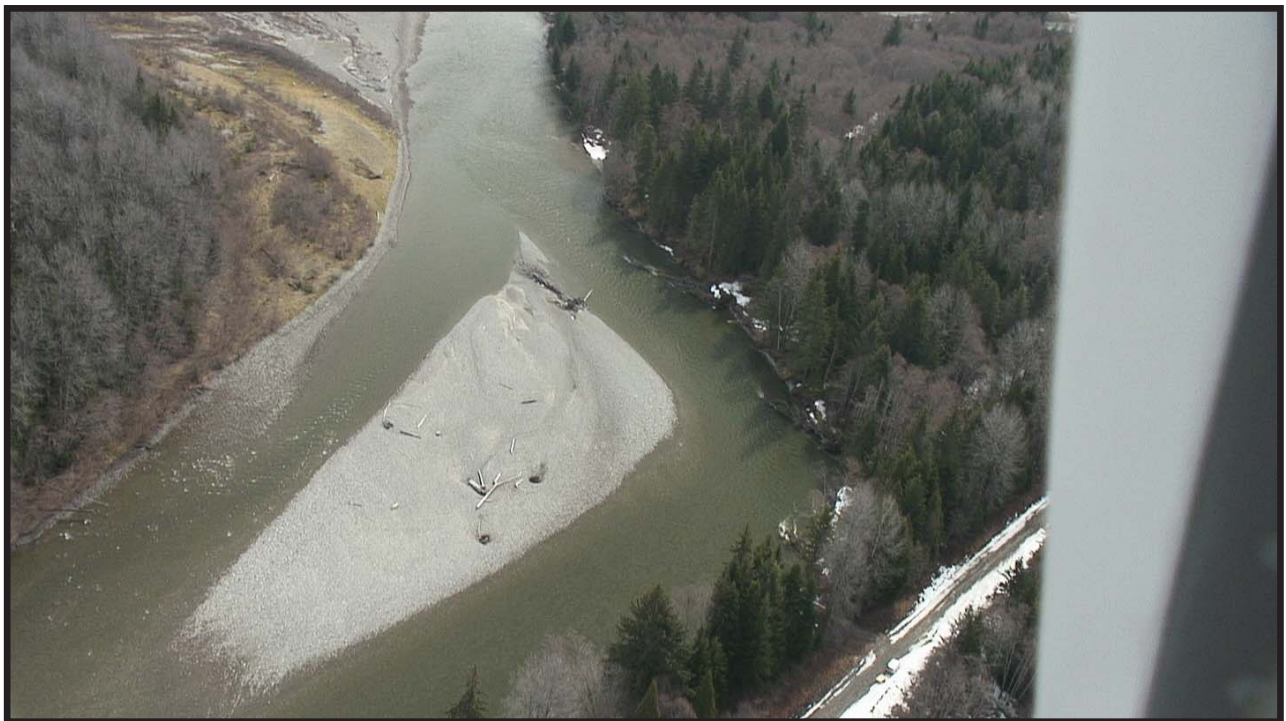
b) Looking downstream to the developing bar and eroding bend.
