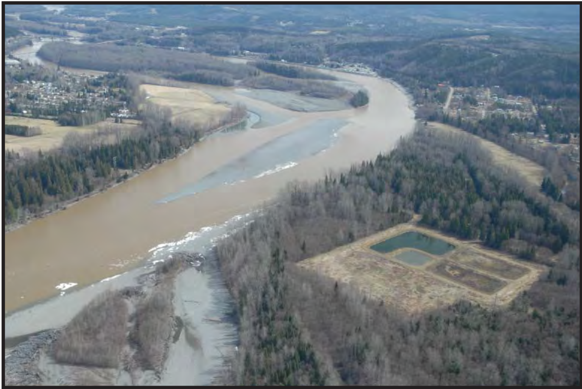
a) Looking upstream illustrating the enlarging gravel bars which are forcing the south channel of Skeena River towards the Regional District STP.
